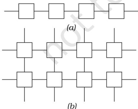
**Fig. 3.6 :** (a) Linear (b) Cross-linked arrangements
